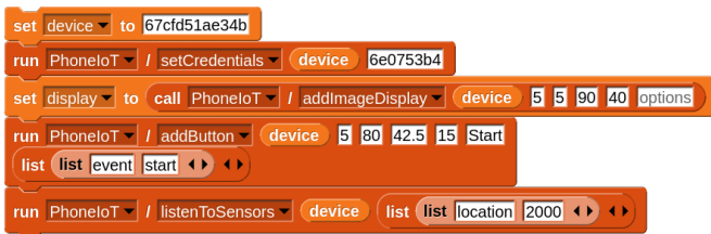
Fig. 5: NetsBlox code to initialize communication with the PhoneIoT app and add GUI widgets on a mobile device
